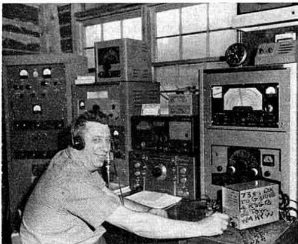
Tom Moss, W4HYW, is the A.R.R.L. W4-K4 QSL Manager but still finds time to do a little operating and is number one in the Award Hunters' Club. Equipment in this picture includes a 500 watt c.w./a.m./s.s.b. transmitter usually operated on 28 Mc/s. The receivers are a National HRO50T1 and Hallicrafters S40A with R.M.E. DB22A preselector and selectoject. The c.w. rig, not shown in this picture, has separate finals for each band from 1.8 to 144 Mc/s. An RTTY position is in process of completion. W4HYW is one of the few U.S. operators to have obtained the Empire DX Certificate.
