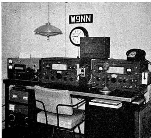
W9NN of Des Plaines, Illinois, operates principally on 7 Mc/s c.w. and has 154 countries confirmed on the band. His equipment includes a Collins 75A1 receiver, 32V1 transmitter and a Viking Thunderbolt. The aerials are a 7 Mc/s dipole and a multiband vertical.
