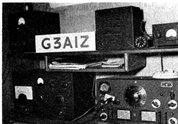
Charles Olley (G3AIZ) of Ilford, Essex, operates from a 6 x 4 ft. "hole in the wall" shack, and has EDXC and WAS for phone operation and 202 countries confirmed for DXCC. The power input is 45 watts to a GSRV type transmitter. The receiver is an HRO and the aerial a home built G4ZU Minibeam at 30 ft.
