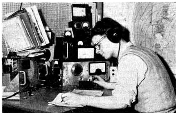
Keith Taylor, G3NNW, who is 17 years of age, operates from his home in Heywood, Lancashire, with the gear shown in this picture. The entire Top Band rig cost only £7. From left to right, the equipment includes an R208 used for DX listening and a BC455 Command receiver used for Top Band (on top of which are the loudspeaker and a clock). The transmitter comprises a v.f.o. for 80 and 160m in the lower rack with the p.a. in the upper one. On top of the transmitter is the aerial current meter and an absorption wavemeter. Other items are a station control unit containing the send/receive switch and indicating lights and a 100/10 kc/s crystal controlled frequency meter. A 10 watt stabilized power supply for the transmitter and various other supplies are located under the table. A 110 ft. end-fed wire aerial is used for Top Band and a 20m dipole with the R208
